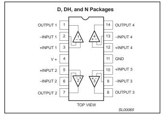
Figure 1. Pin configuration.
