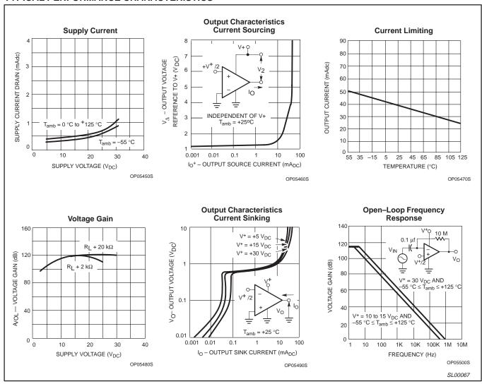
Figure 3. Typical Performance Characteristics
